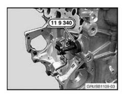
Fit the chain tensioner (Special Tool 11 9 340) without the seal ring and with the lock nut loose. Pretension the chain tensioner with Special Tool 00 9 250 to 0.6 Nm. Finger-tighten the lock nut on Special Tool 11 9 340.
